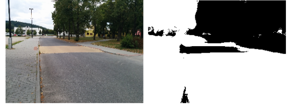
Fig. 9: Applying a \leq 40 saturation threshold on a street image.
