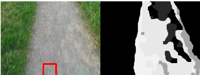
Fig. 4: Backprojection of a reference region (marked in red on the left) into the image (left). The resulting probabilities in grayscale (right).
