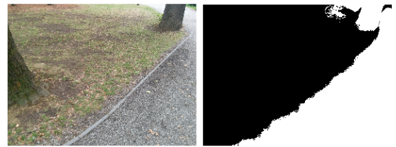
Fig. 10: Applying a \leq 40 saturation threshold on a transition situation.
