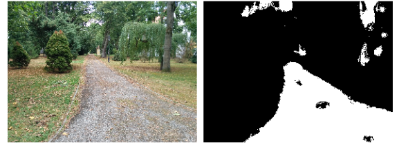
Fig. 8: Applying a \leq 40 saturation threshold on a park image.
